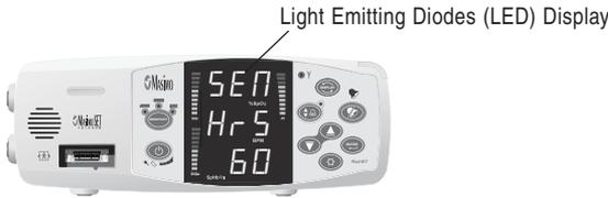
The Rad-87 LED displays messages to communicate the remaining sensor time available to the user, as defined in the following table:
