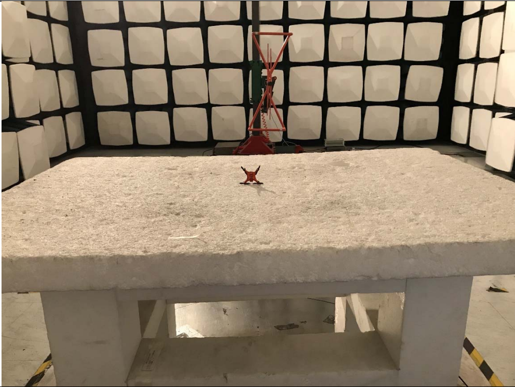
Radiated emission Test Setup-1 (30 MHz~1 GHz)
