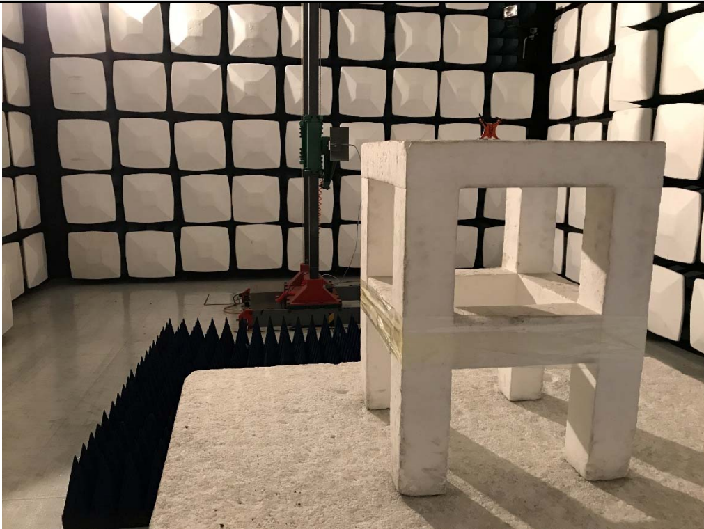
Radiated emission Test Setup-2 (Above 1 GHz)
