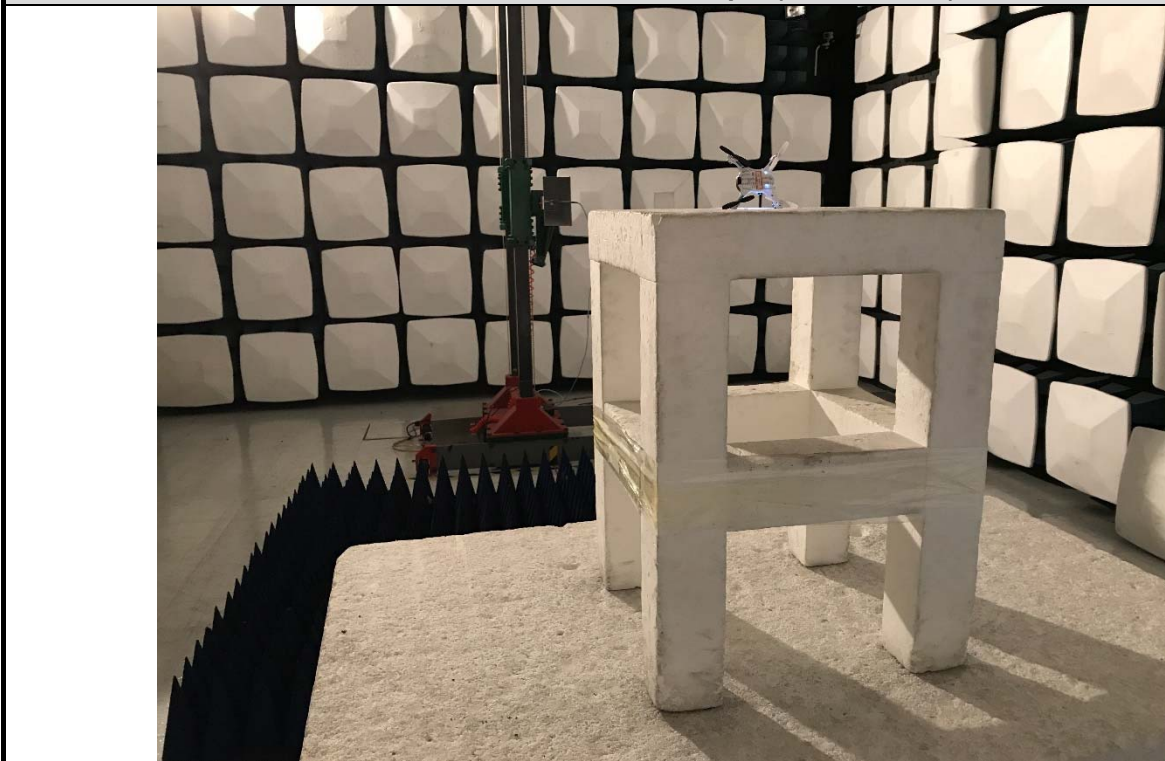
Radiated emission Test Setup-2 (Above 1 GHz)
