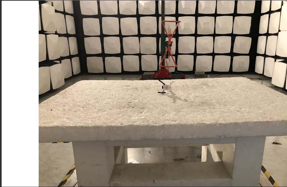
Radiated emission Test Setup-1 (30 MHz~1 GHz)
