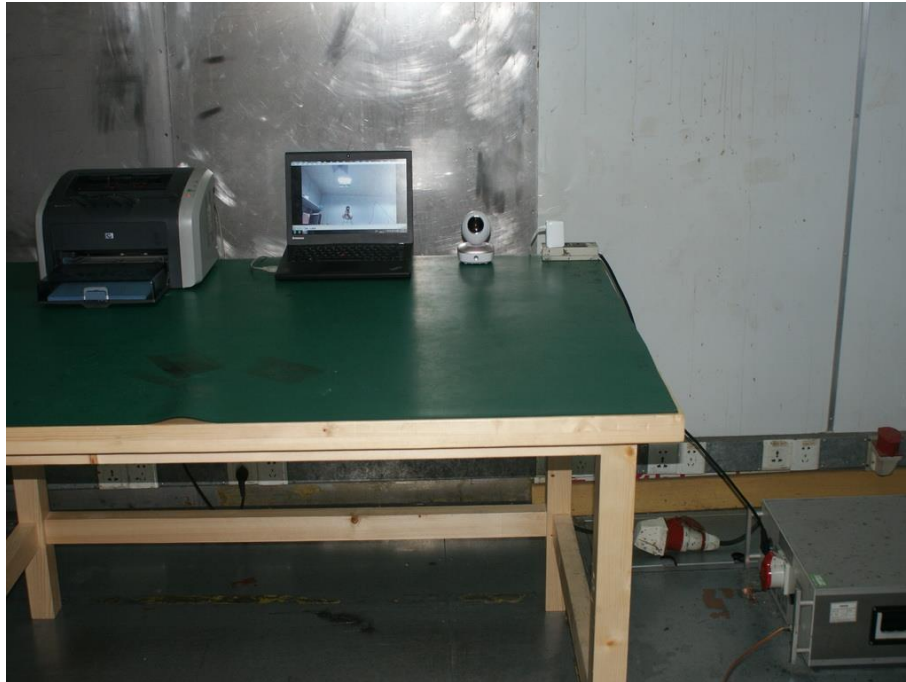
Photograph 2: Set-up for Radiated Emission (30MHz ~ 1GHz)
