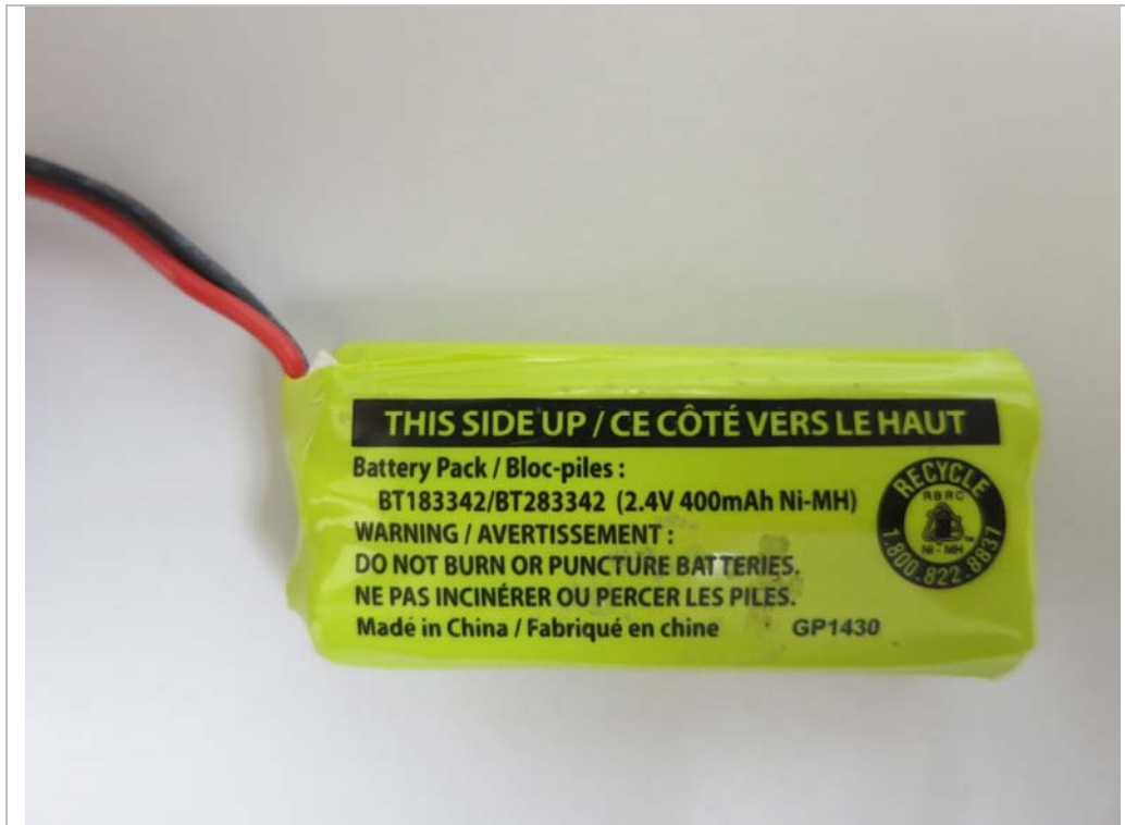
Figure 3 – 2.4V 400mAh Ni-MH GPI rechargeable battery front view
