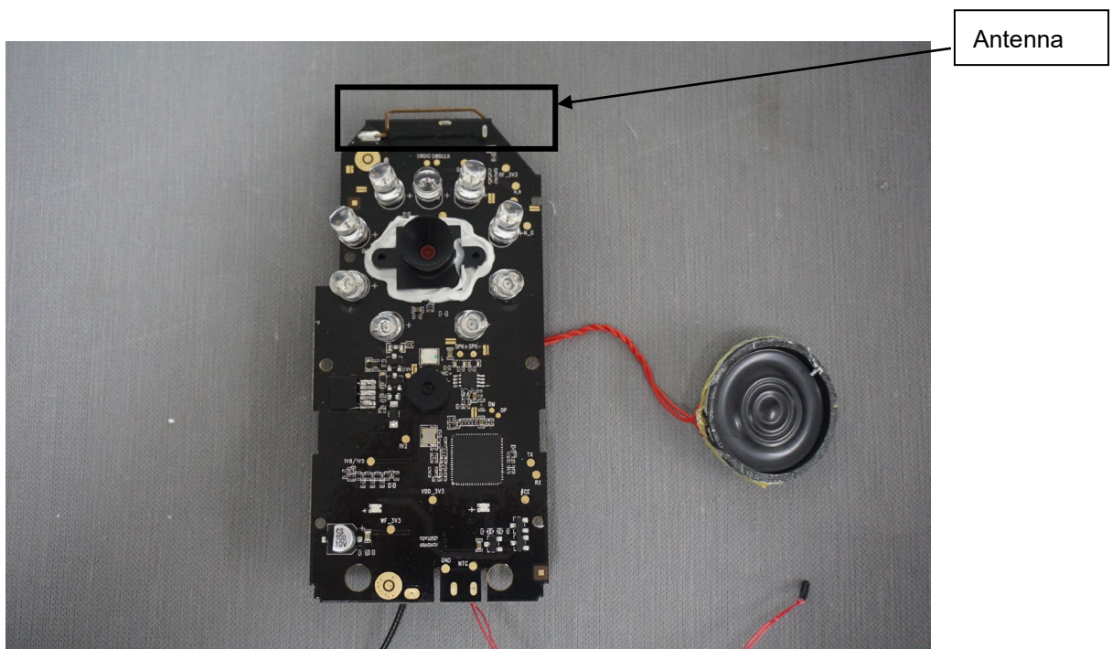
Photo of antenna refer to Appendix – Internal photo.
