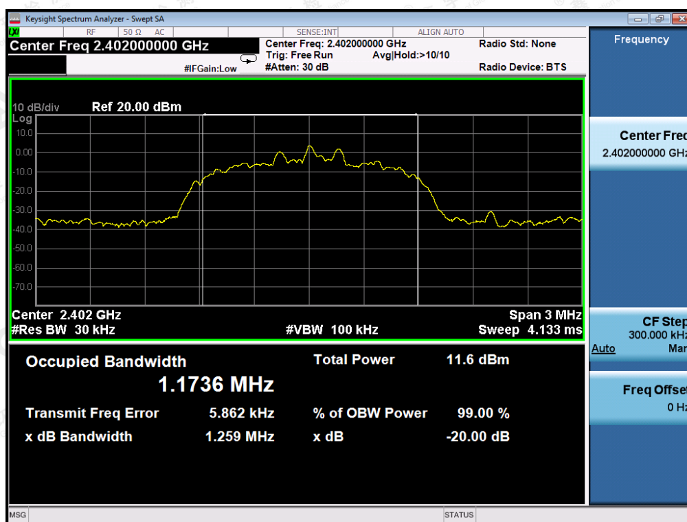
TEST PLOT OF BANDWIDTH FOR LOW CHANNEL
