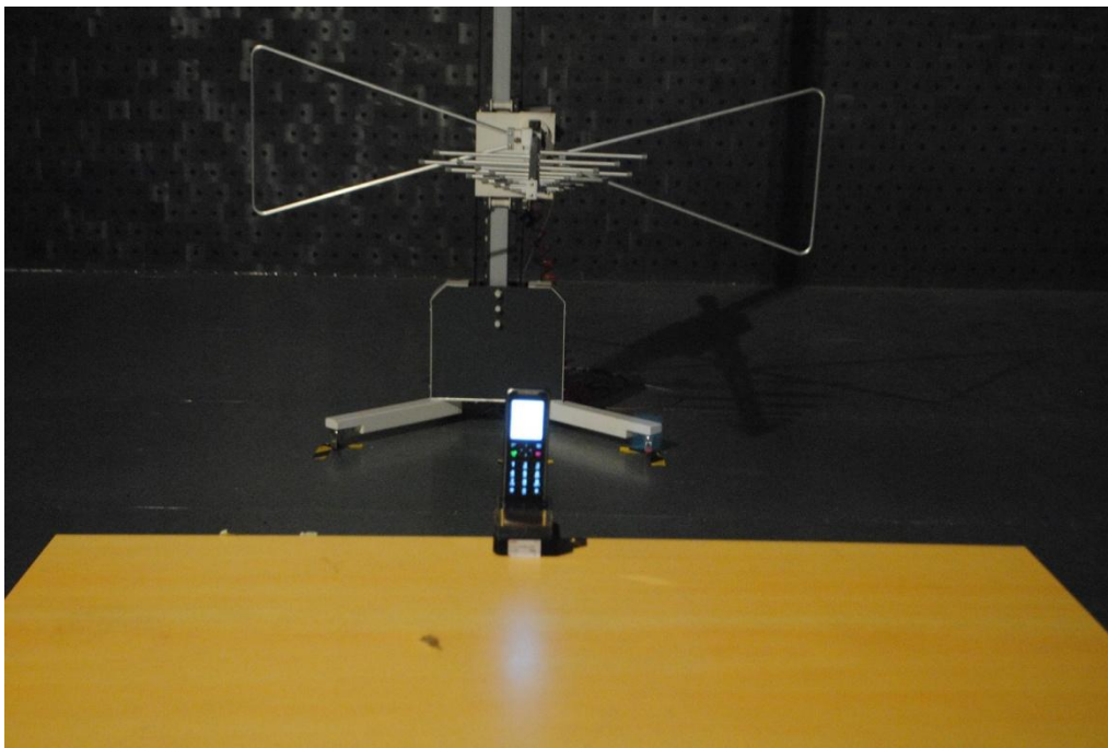
PP Radiated Emission test view (Frequency from 30MHz to 1GHz)
