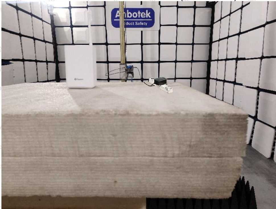
Photo of Radiation Emission Test (above 1GHz)
