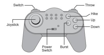
JOYSTICK - drives the robot forward, backward, and turns. Joystick control is PROPORTIONAL. This means the further you push the joystick in one direction, the FASTER it goes. Small motions on the joystick get small controlled motions on the robot.
