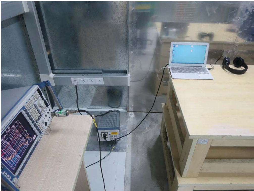
FCC RADIATED EMISSION TEST SETUP
