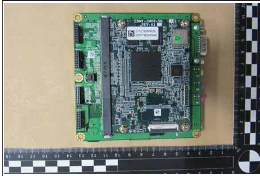
AE 1: Wandboard WBIMX6U, Bottom View
