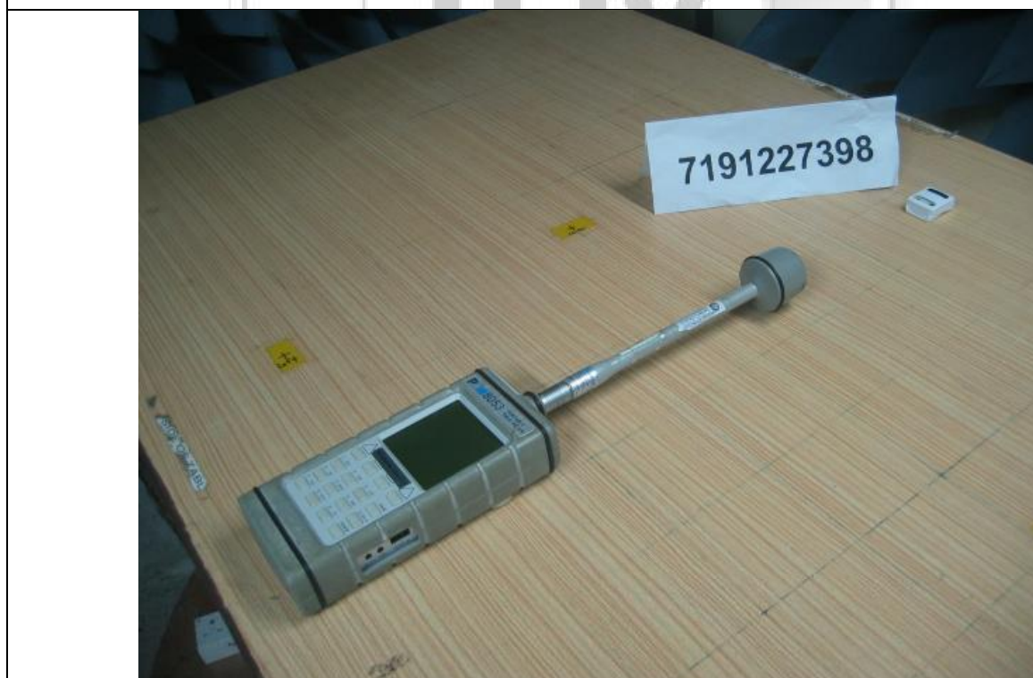
Maximum Permissible Exposure (MPE) Test Setup
