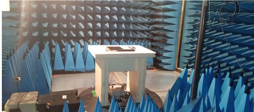
Test setup in anechoic chamber – Frequency >1GHz
