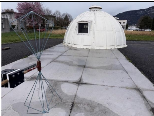
Test setup of Field strength within the band 13.110-14.010MHz in OATS
