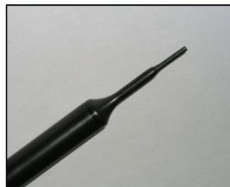
EX3DV4 E-field Probe
