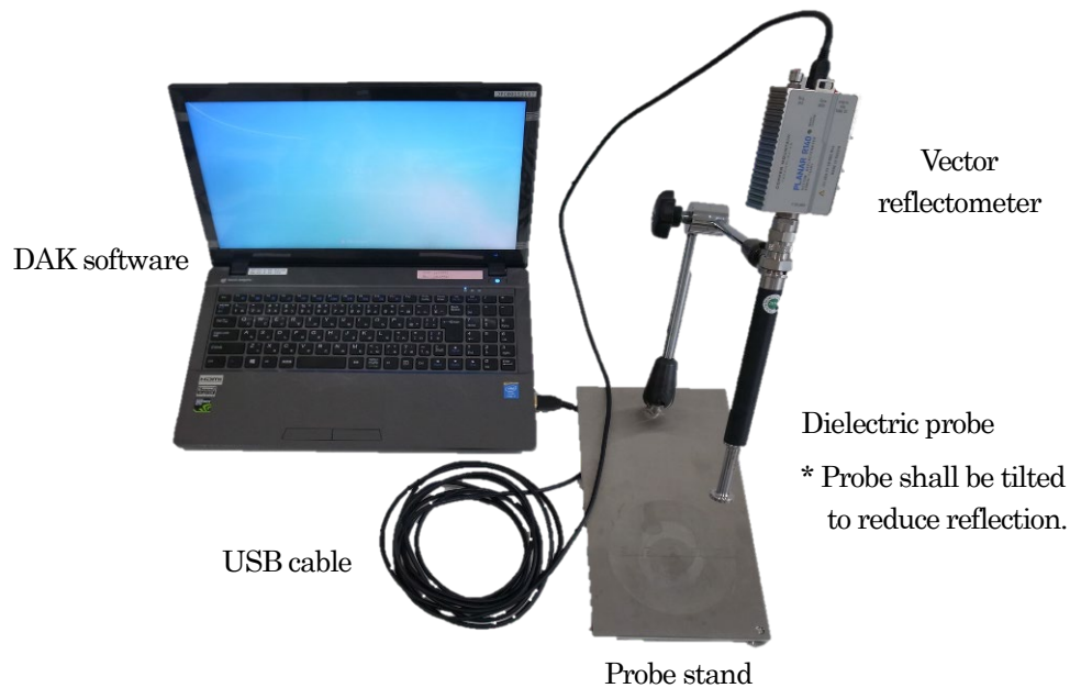
(a) Dielectric Parameter Measurement System
