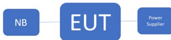
Fig. 2-2 Conducted (Antenna Port) Configuration
