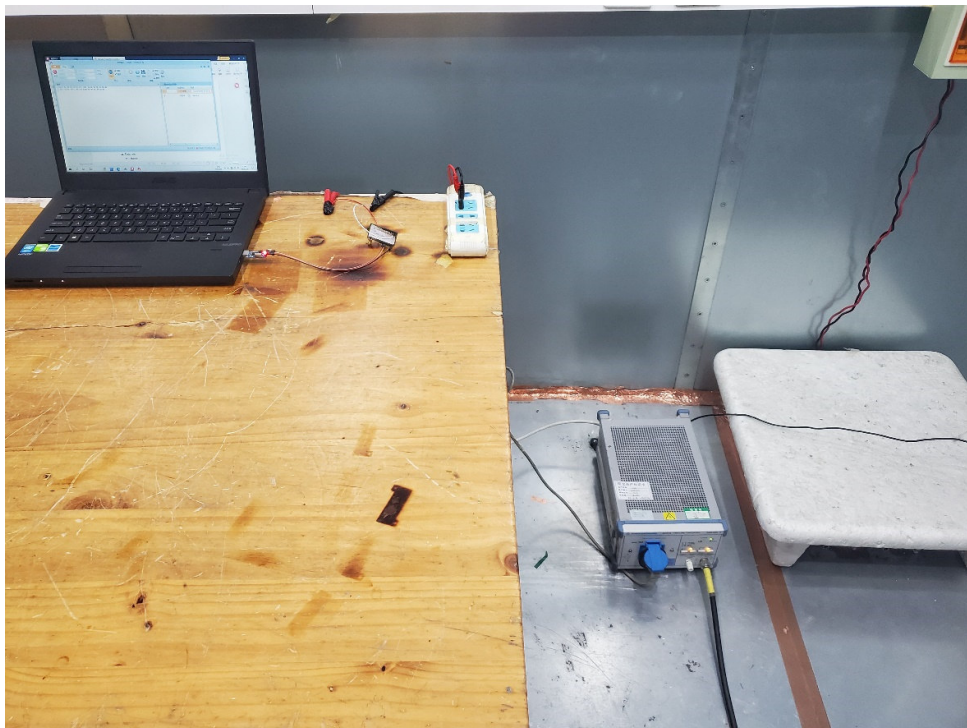
Picture 2 Conducted Emission Test Setup
