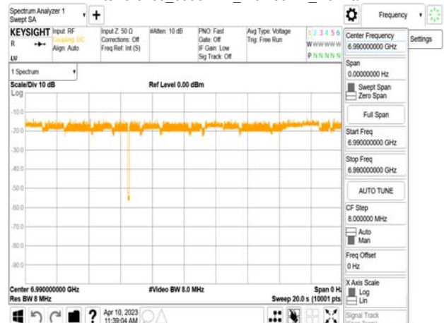
802.11ax_80MHz_CF 7025MHz_ Interference_6990MHz_-76.73dBm_Normal
