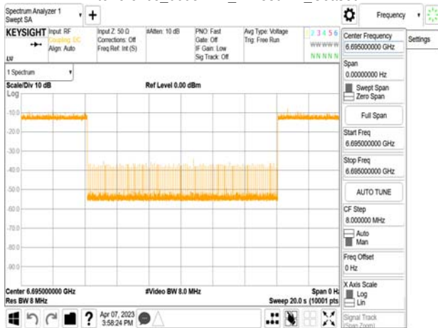
802.11ax_20MHz_CF 6695MHz_ Interference_6695MHz_-74.74dBm_Minimal
