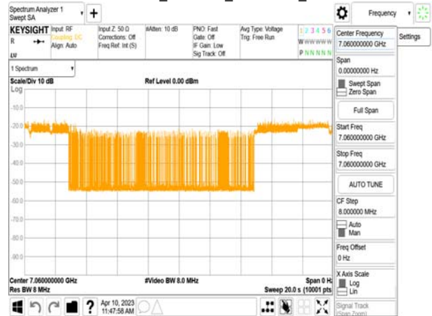
802.11ax_80MHz_CF 7025MHz_ Interference_7060MHz_-76.77dBm_Normal
