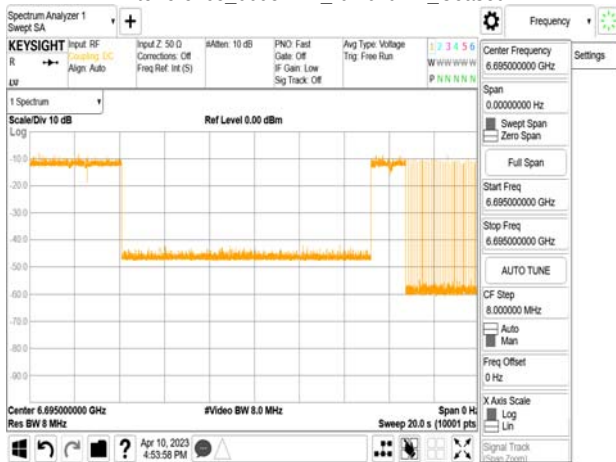
802.11ax_20MHz_CF 6695MHz_ Interference_6695MHz_-73.62dBm_Minimal
