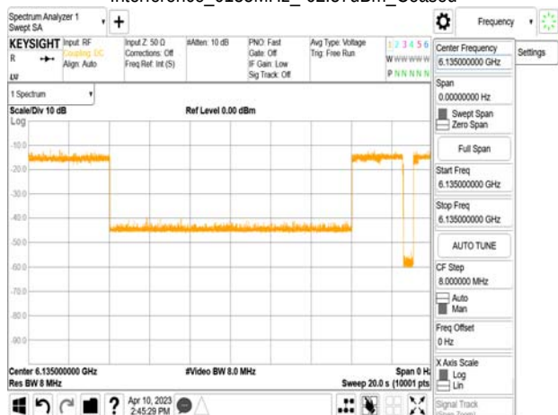
802.11ax_20MHz_CF 6135MHz_ Interference_6135MHz_-69.57dBm_Minimal
