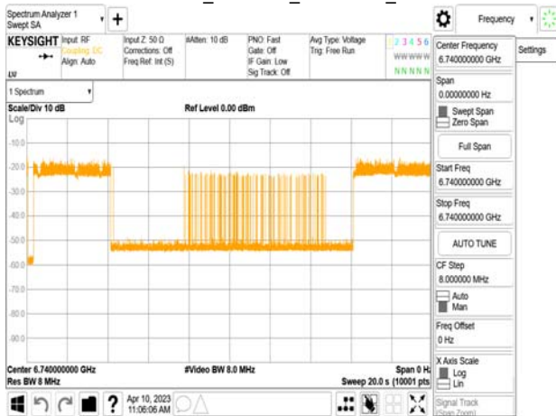
802.11ax_80MHz_CF 6705MHz_ Interference_6740MHz_-73.66dBm_Normal
