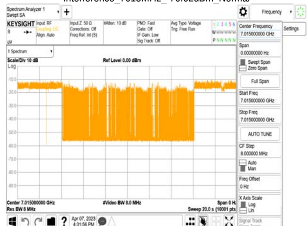
802.11ax_20MHz_CF 7015MHz_ Interference_7015MHz_-76.62dBm_Normal
