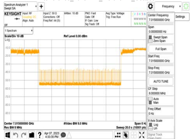
802.11ax_20MHz_CF 7015MHz_ Interference_7015MHz_-76.12dBm_Minimal
