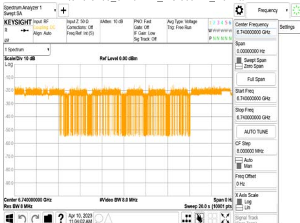
802.11ax_80MHz_CF 6705MHz_ Interference_6740MHz_-73.66dBm_Normal
