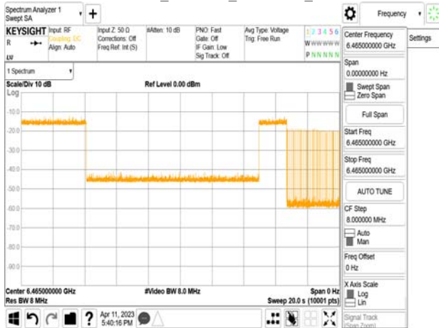
802.11ax_80MHz_CF 6465MHz_ Interference_6465MHz_-67.85dBm_Minimal
