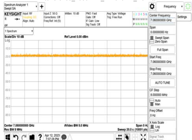
802.11ax_80MHz_CF 7025MHz_ Interference_7060MHz_-74.61dBm_Normal
