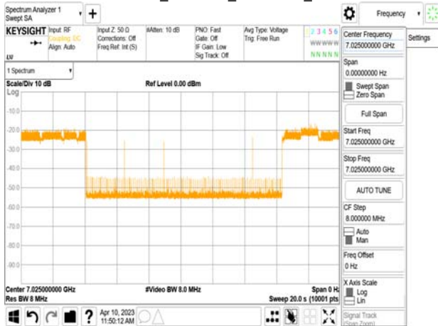
802.11ax_80MHz_CF 7025MHz_ Interference_7025MHz_-76.52dBm_Normal
