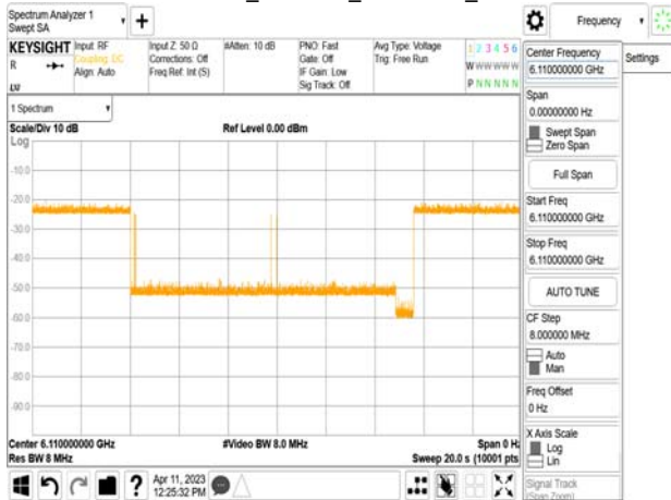
802.11ax_80MHz_CF 6145MHz_ Interference_6110MHz_-70.69dBm_Normal
