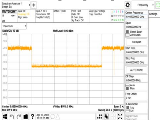
802.11ax_80MHz_CF 6465MHz_ Interference_6465MHz_-67.64dBm_Minimal
