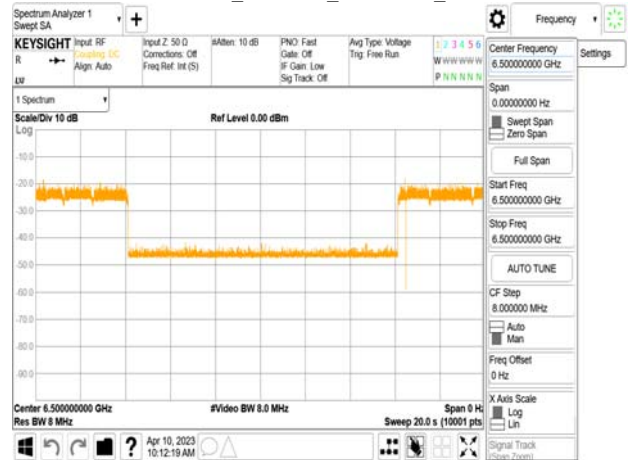
802.11ax_80MHz_CF 6465MHz_ Interference_6500MHz_-67.67dBm_Minimal
