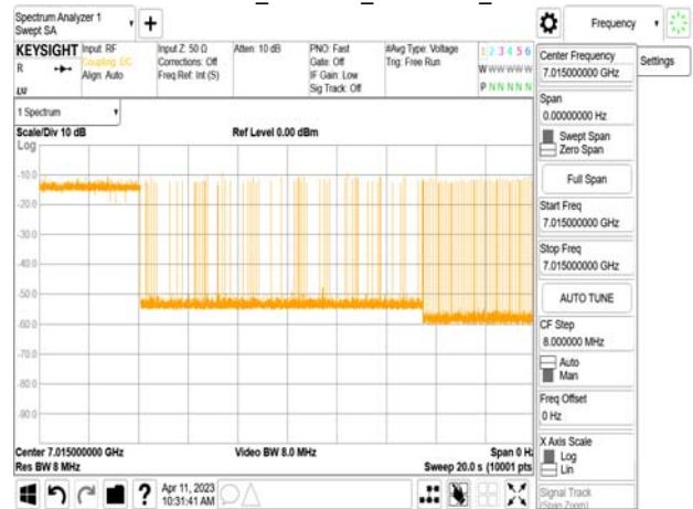
802.11ax_20MHz_CF 7015MHz_ Interference_7015MHz_-76.52dBm_Normal
