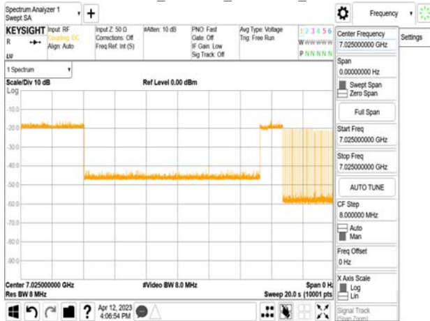
802.11ax_80MHz_CF 7025MHz_ Interference_7025MHz_-74.72dBm_Minimal
