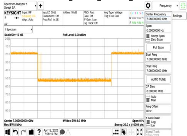
802.11ax_80MHz_CF 7025MHz_ Interference_7060MHz_-74.61dBm_Normal
