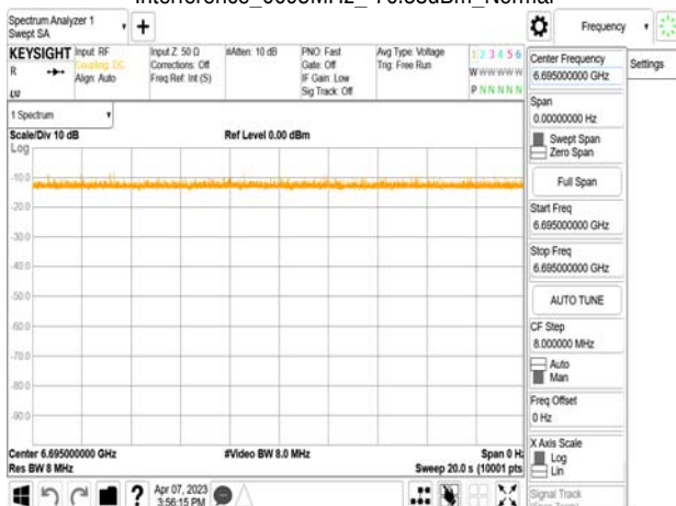
802.11ax_20MHz_CF 6695MHz_ Interference_6695MHz_-76.53dBm_Normal
