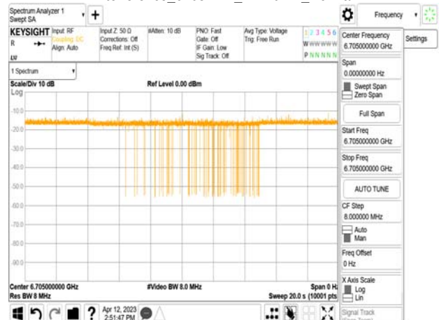
802.11ax_80MHz_CF 6705MHz_ Interference_6705MHz_-74.7dBm_Normal
