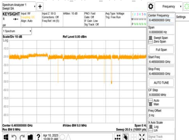
802.11ax_80MHz_CF 6465MHz_ Interference_6465MHz_-70.64dBm_Normal
