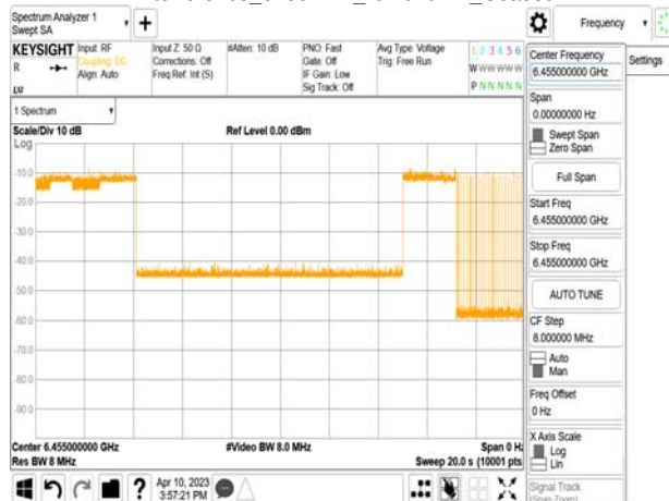
802.11ax_20MHz_CF 6455MHz_ Interference_6455MHz_-67.62dBm_Minimal
