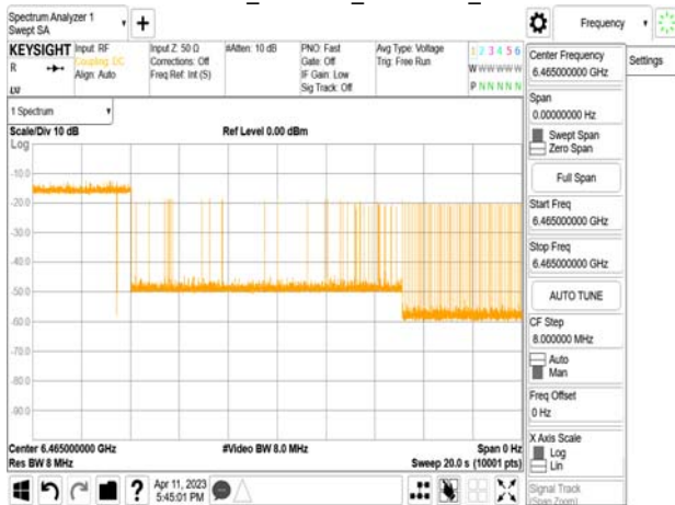
802.11ax_80MHz_CF 6465MHz_ Interference_6465MHz_-70.85dBm_Normal
