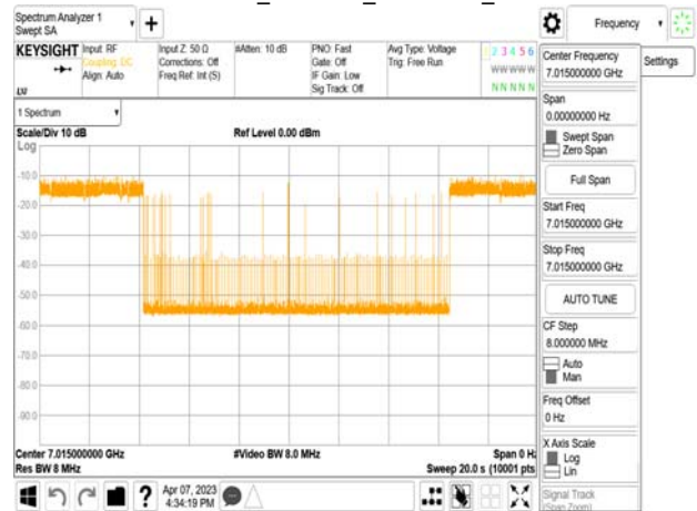
802.11ax_20MHz_CF 7015MHz_ Interference_7015MHz_-76.62dBm_Normal
