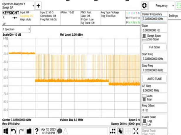
802.11ax_80MHz_CF 7025MHz_ Interference_7025MHz_-77.72dBm_Normal
