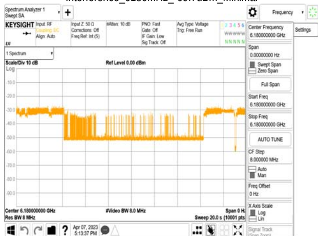
802.11ax_80MHz_CF 6145MHz_ Interference_6180MHz_-70.7dBm_Normal
