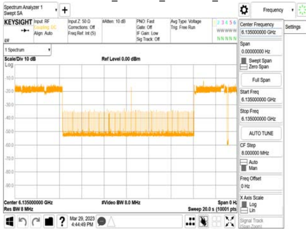
802.11ax_20MHz_CF 6135MHz_ Interference_6135MHz_-73.83dBm_Normal
