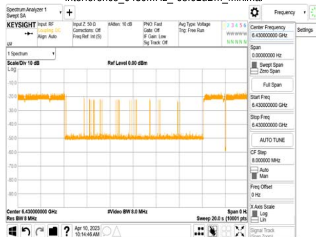
802.11ax_80MHz_CF 6465MHz_ Interference_6430MHz_-70.61dBm_Normal
