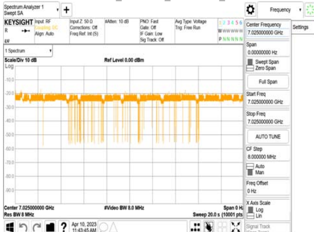
802.11ax_80MHz_CF 7025MHz_ Interference_7025MHz_-76.52dBm_Normal
