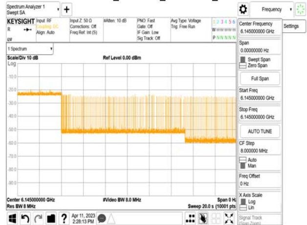
802.11ax_80MHz_CF 6145MHz_ Interference_6145MHz_-73.56dBm_Normal
