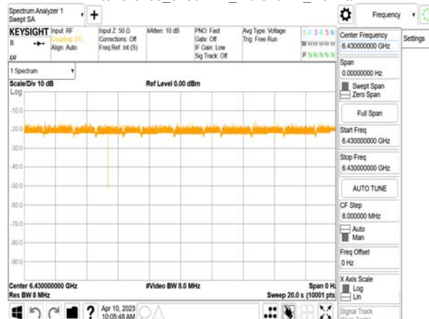
802.11ax_80MHz_CF 6465MHz_ Interference_6430MHz_-70.61dBm_Normal
