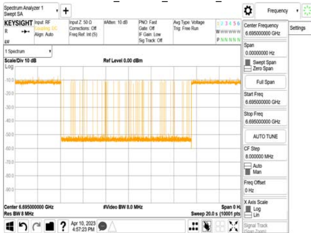
802.11ax_20MHz_CF 6695MHz_ Interference_6695MHz_-76.62dBm_Normal
