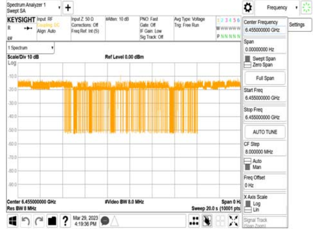
802.11ax_20MHz_CF 6455MHz_ Interference_6455MHz_-70.64dBm_Normal
