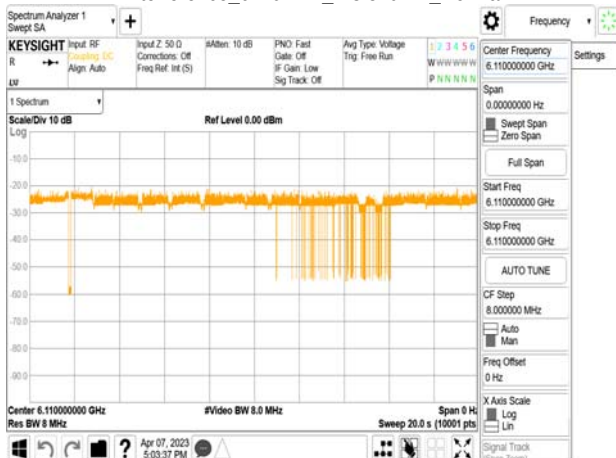
802.11ax_80MHz_CF 6145MHz_ Interference_6110MHz_-73.51dBm_Normal
