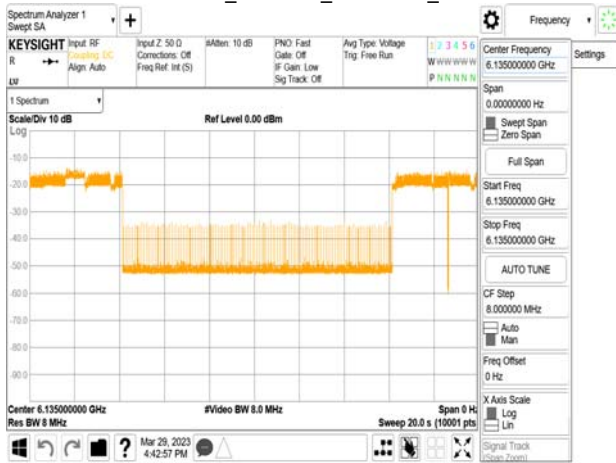
802.11ax_20MHz_CF 6135MHz_ Interference_6135MHz_-71.83dBm_Minimal
