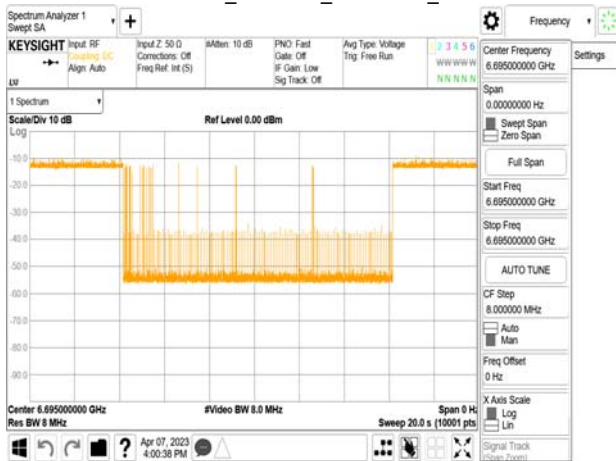
802.11ax_20MHz_CF 6695MHz_ Interference_6695MHz_-76.53dBm_Normal
