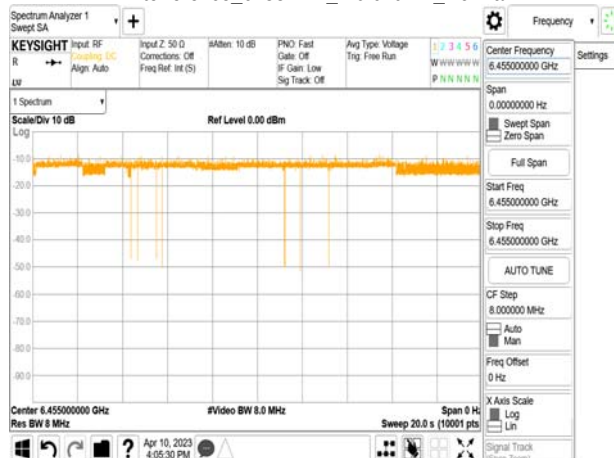
802.11ax_20MHz_CF 6455MHz_ Interference_6455MHz_-70.62dBm_Normal
