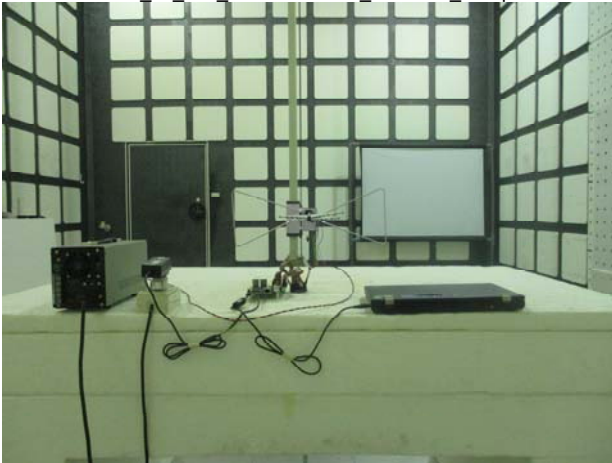
Part 15 247 IEEE 802.15.4 Radiated Setup
