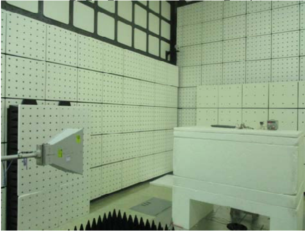
Part 15 247 IEEE 802.15.4 Radiated Setup
