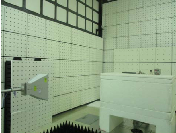
Part 15 407 WLAN 5G Radiated Setup
