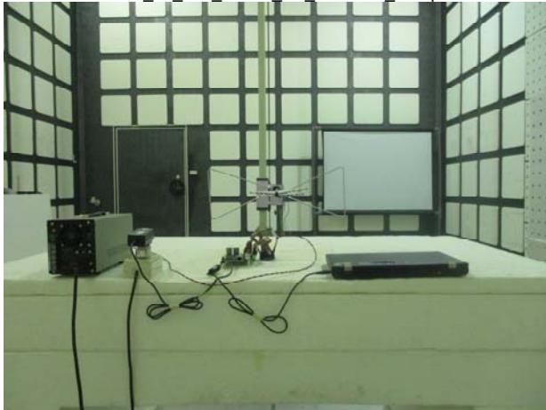
Part 15 407 WLAN 5G Radiated Setup
