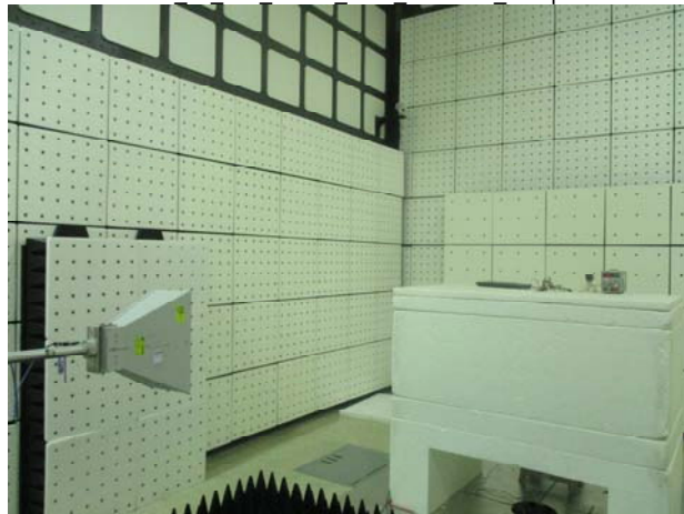
Part 15 247 WLAN 2.4G Radiated Setup
