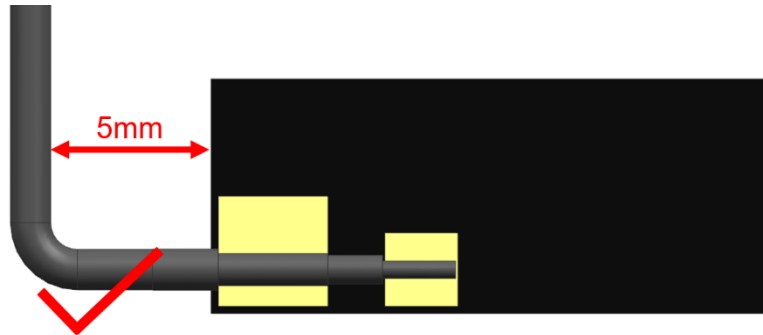
FIGURE 5.2.1 RECOMMENDED CABLE BENDING RANGE
