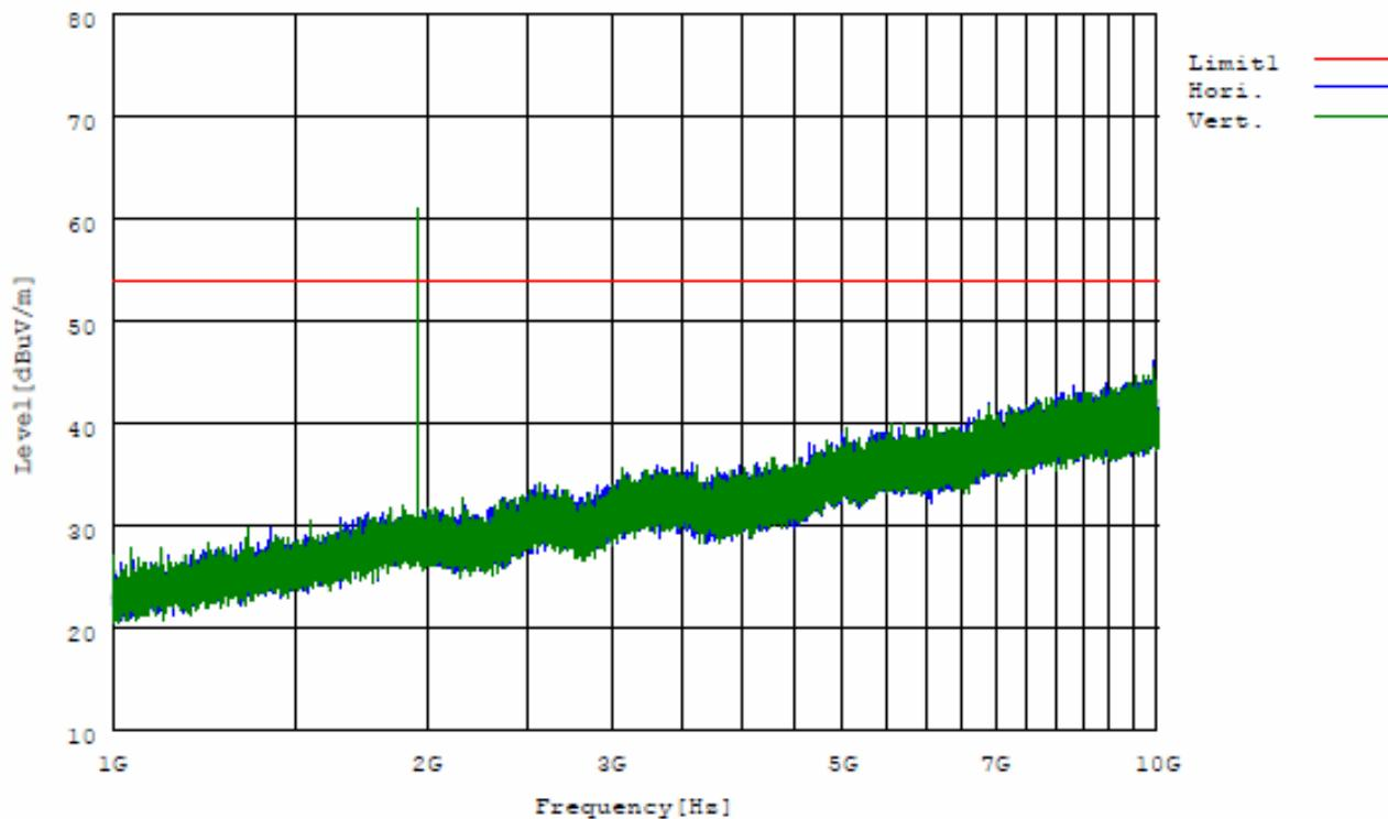
Note : A spectrum @1954MHz is downlink signal from RF tester. This is used to set EUT in idle mode. This is not a spurious emission from EUT.
