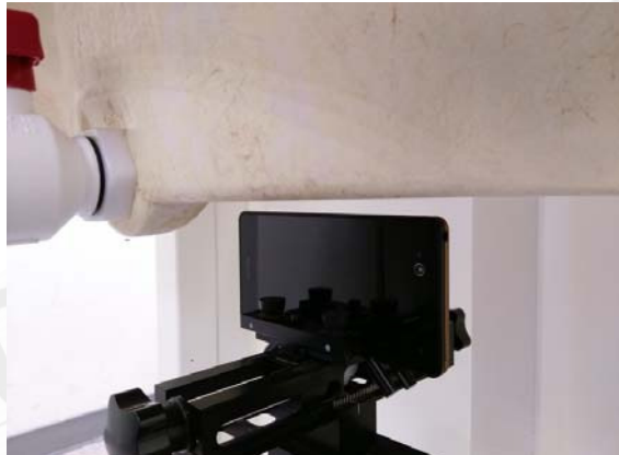
Fig.13 EUT Left side to flat phantom
