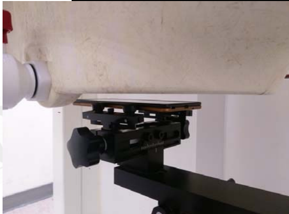
Fig.9 EUT Front side to flat phantom
