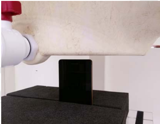
Fig.10 EUT Bottom side to flat phantom
