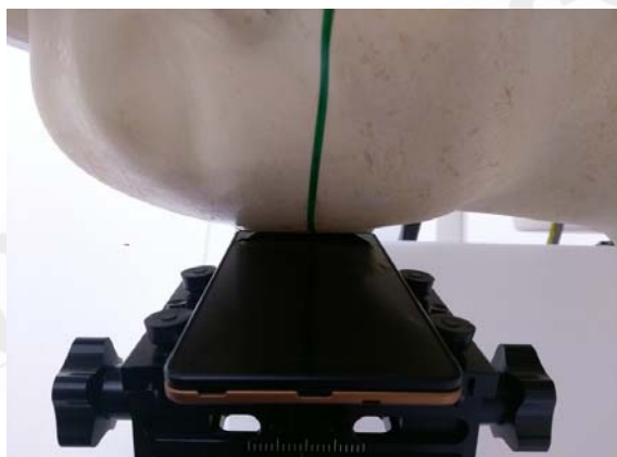
Fig.4 Right Head Section / Ear-Tilt Position(15°)
