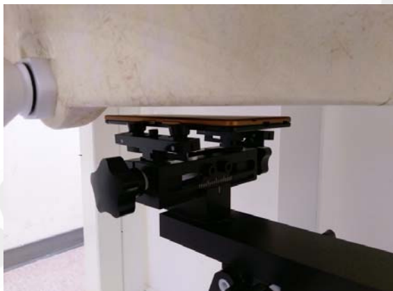
Fig.11 EUT Back side to flat phantom
