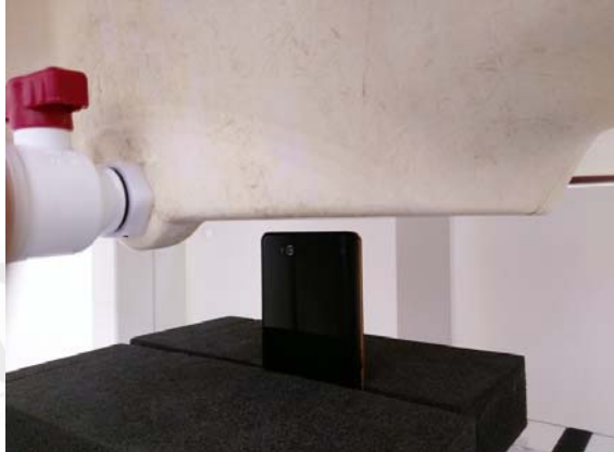
Fig.12 EUT Top side to flat phantom
