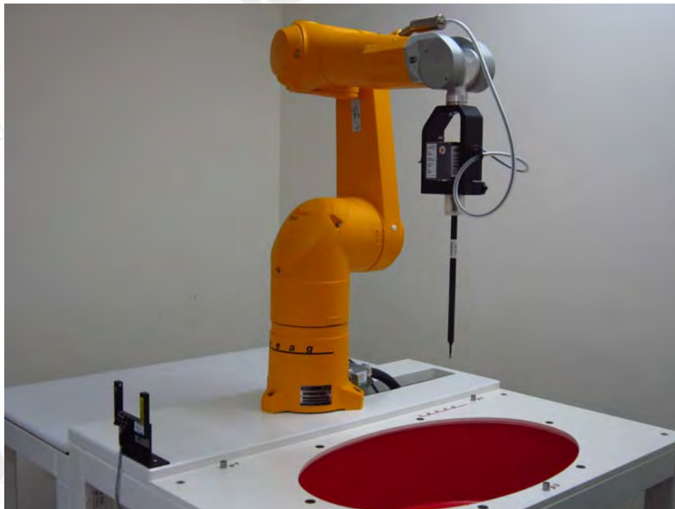
Fig.1 Photograph of the SAR measurement system
