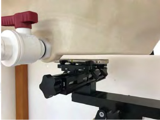
Fig.9 EUT Front side to flat phantom
