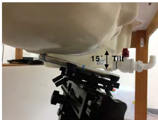
Fig.4 Right Head Section / Ear-Tilt Position(15°)
