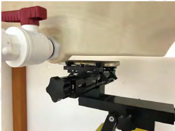
Fig.8 EUT Back side to flat phantom
