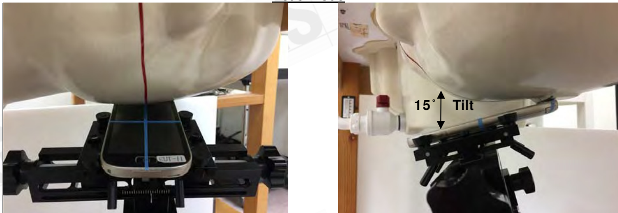
Fig.6 Left Head Section / Ear-Tilt Position(15°)
