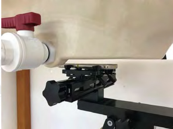
Fig.7 EUT Front side to flat phantom
