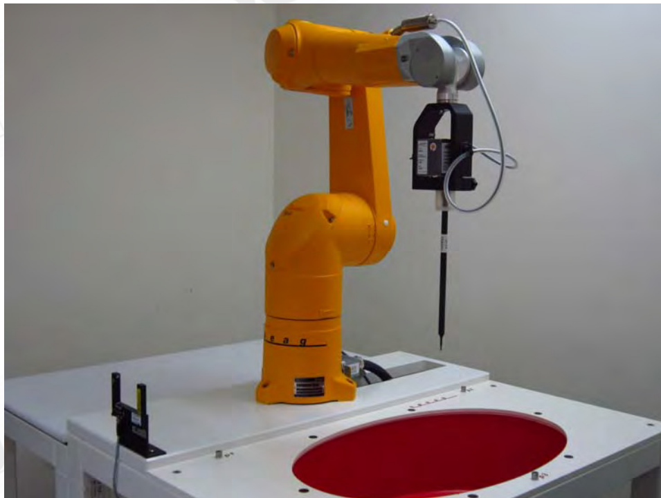
Fig.1 Photograph of the SAR measurement system
