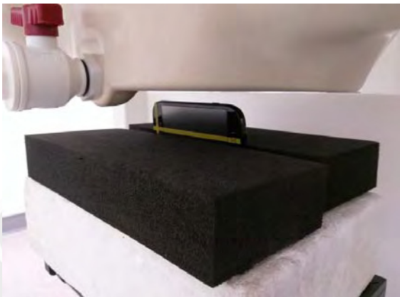
Fig.14 EUT Right side to flat phantom
