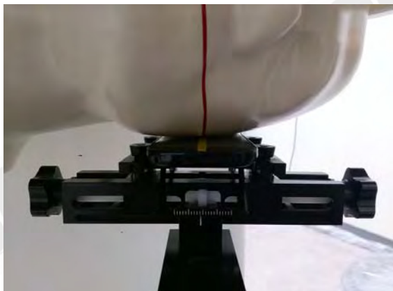
Fig.5 Left Head Section / Cheek-Touch Position
