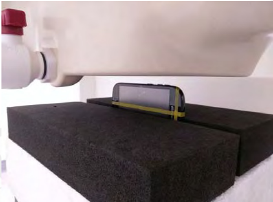
Fig.13 EUT Left side to flat phantom
