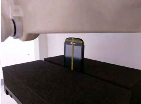
Fig.12 EUT Top side to flat phantom
