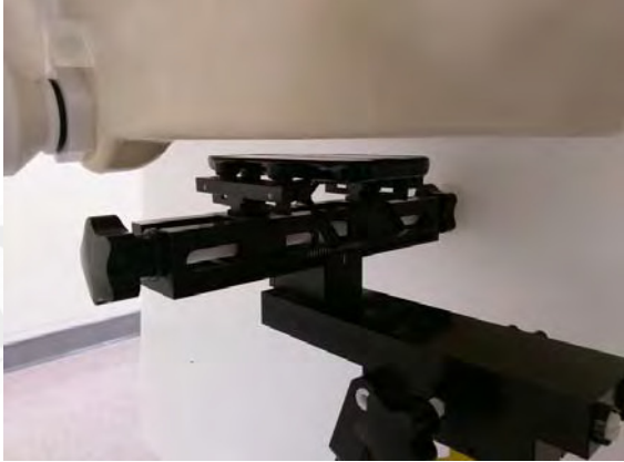
Fig.9 EUT Front side to flat phantom
