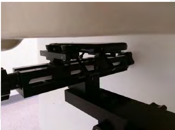
Fig.11 EUT Back side to flat phantom
