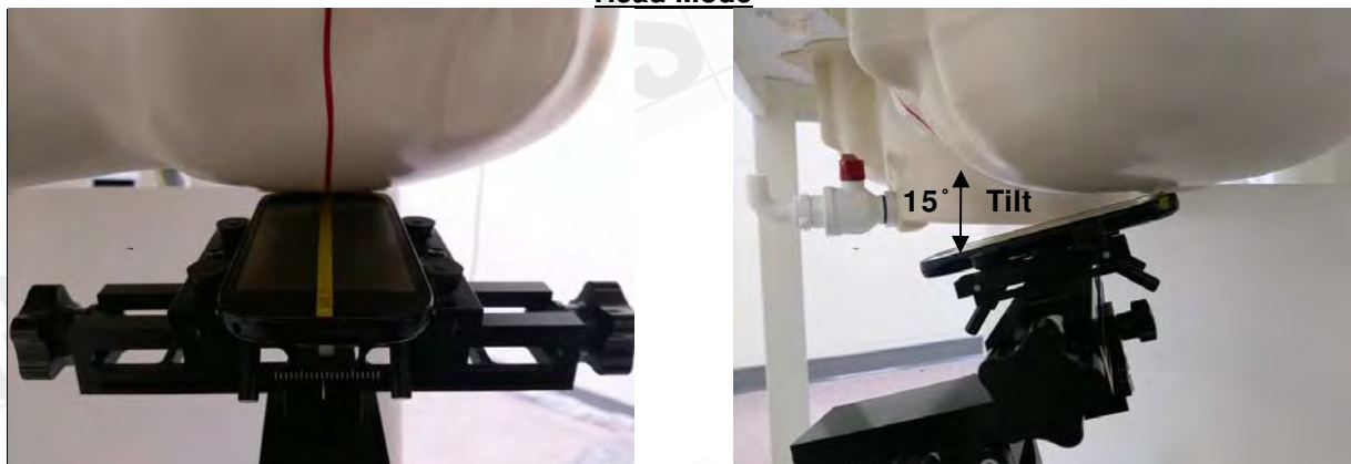
Fig.6 Left Head Section / Ear-Tilt Position(15°)
