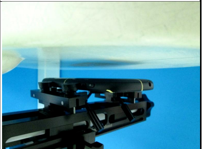
Rear Face of EUT with 1.5 cm Gap
