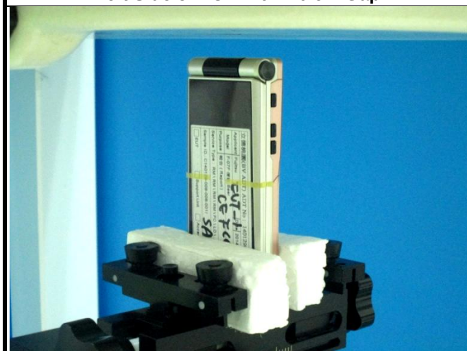
Top Side of EUT with 1.0 cm Gap
