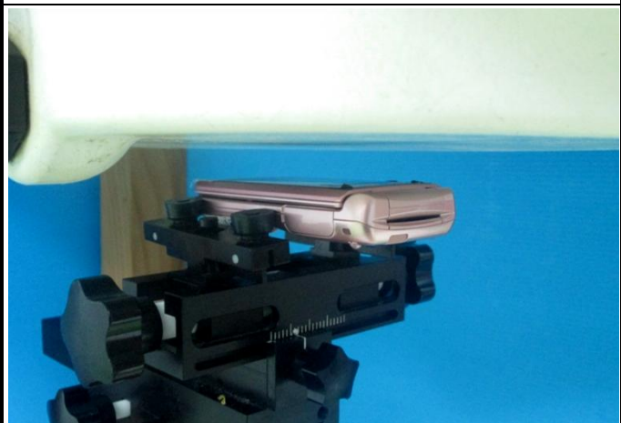
Front Face of EUT with 1.5 cm Gap
