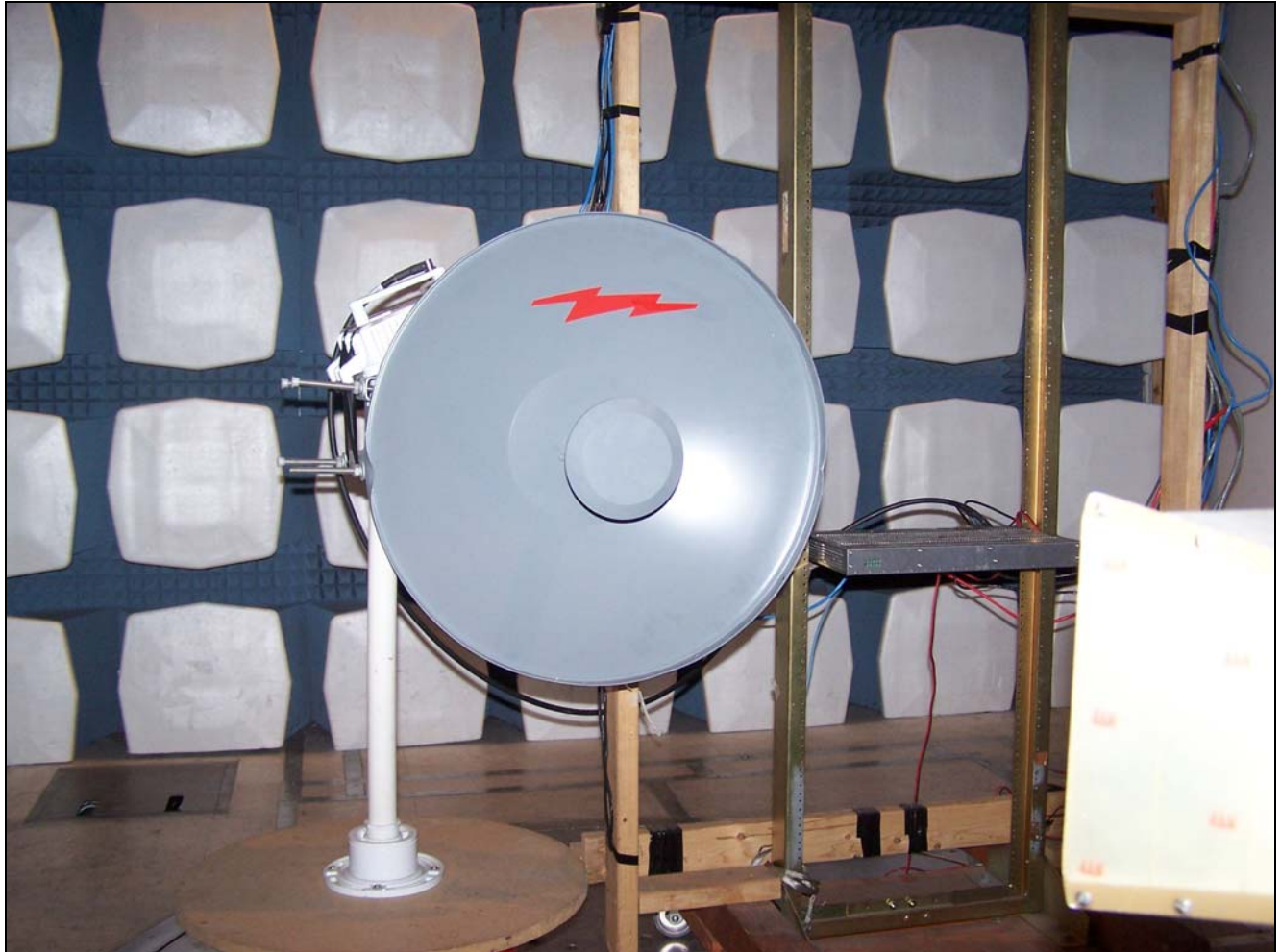
Photograph 3. Radiated Spurious Emissions, Test Setup
