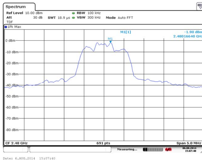
Fig. 46 Conducted Spurious Emission (8DPSK, Ch78, 2.480GHz)
