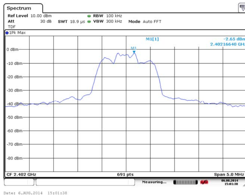
Fig. 40 Conducted Spurious Emission (8DPSK, Ch0, 2.402GHz)
