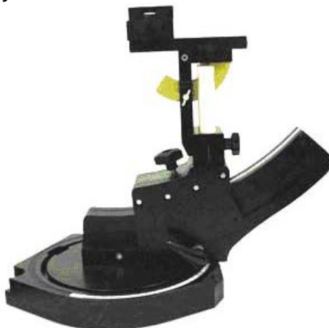
Device holder supplied by SPEAG
