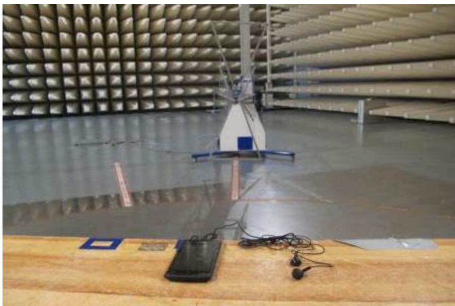
Spurious Radiated Emissions Test setup (30MHz~1GHz)
