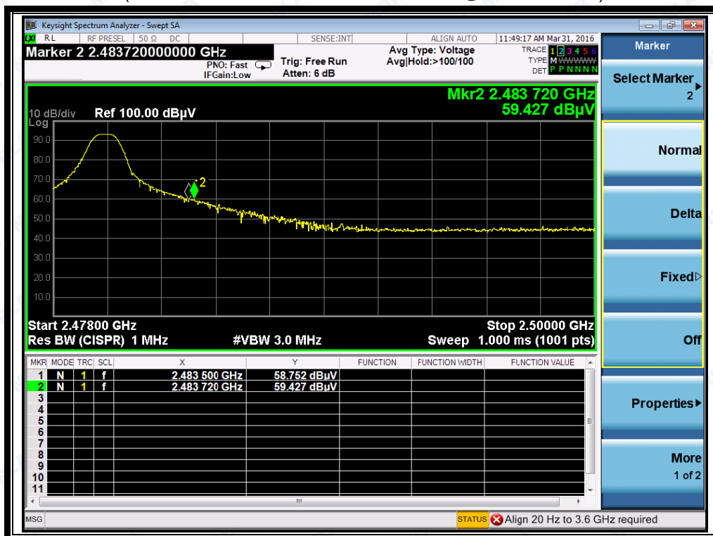
(Plot D1: Channel = 78 PEAK @ \pi/4 -DQPSK)
