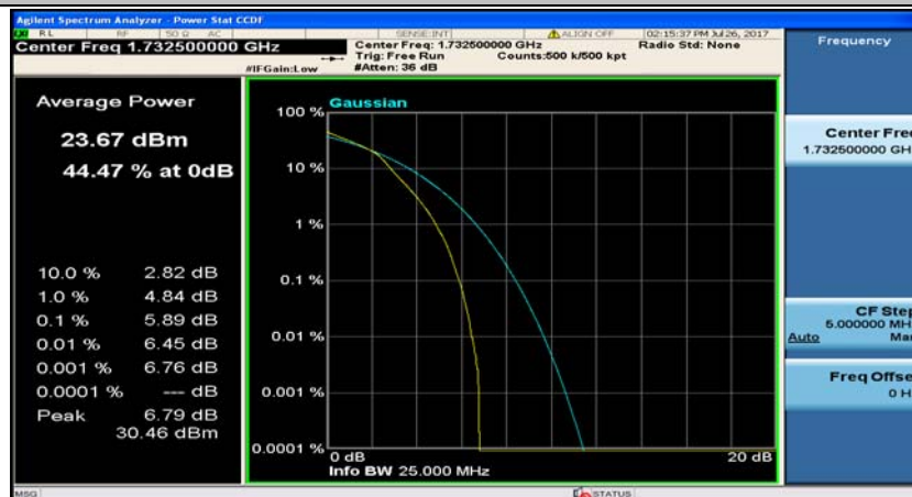
(Channel Bandwidth: 5 MHz)_MCH_16QAM_12RB#13
