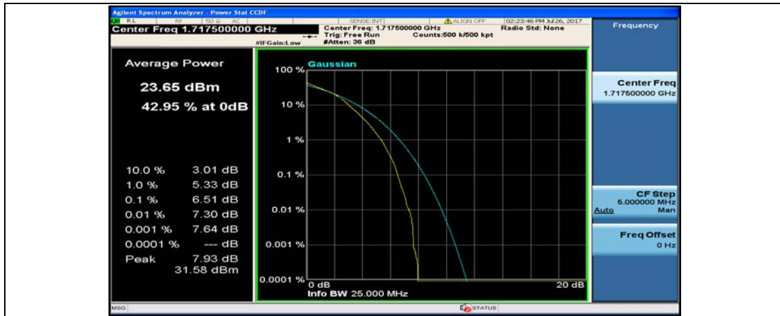
(Channel Bandwidth:15 MHz)_MCH_16QAM_1RB#0
