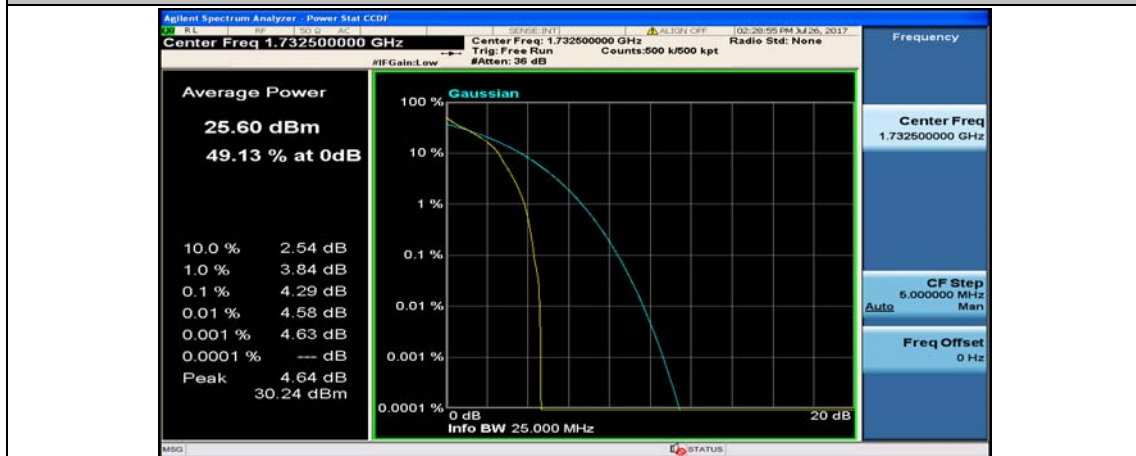
(Channel Bandwidth:20 MHz)_MCH_QPSK_1RB#99
