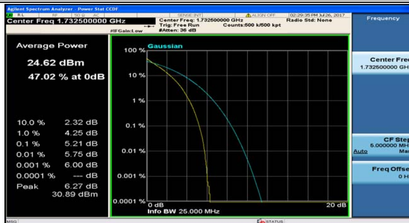
(Channel Bandwidth:20 MHz)_MCH_QPSK_50RB#50
