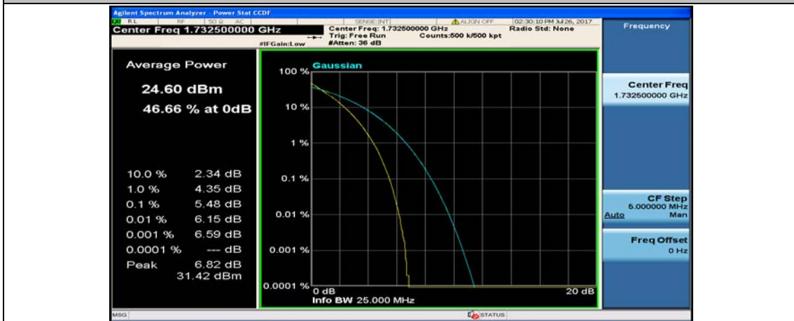
(Channel Bandwidth:20 MHz)_MCH_QPSK_100RB#0
