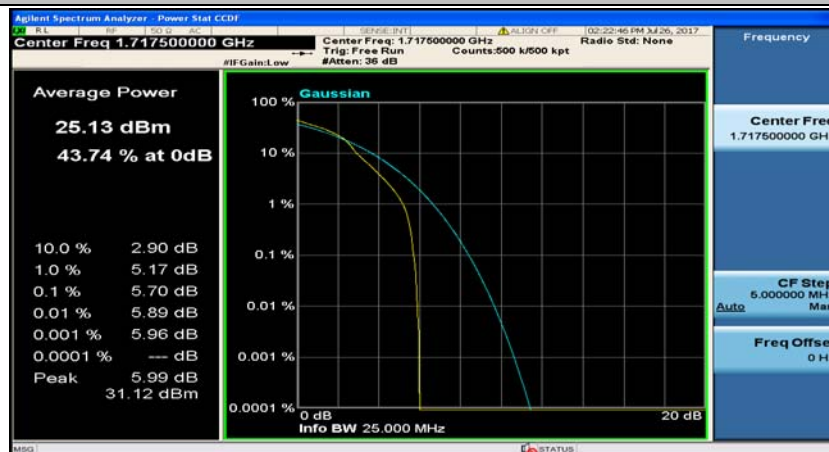
(Channel Bandwidth:15 MHz)_LCH_16QAM_37RB#0
