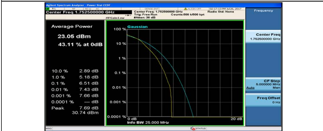
(Channel Bandwidth: 5 MHz)_HCH_16QAM_25RB#0
