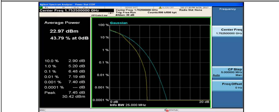
(Channel Bandwidth: 5 MHz)_HCH_16QAM_25RB#0
