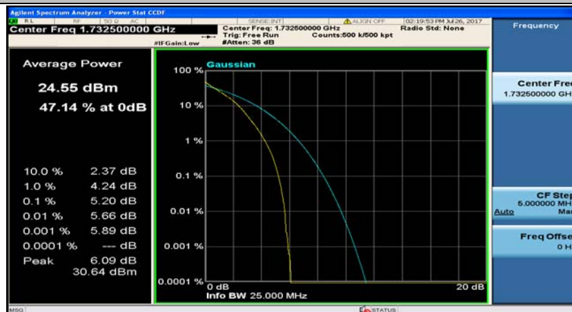
Channel Bandwidth: 10 MHz_MCH_QPSK_25RB#25
