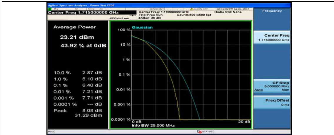
Channel Bandwidth: 10 MHz_MCH_16QAM_1RB#0
