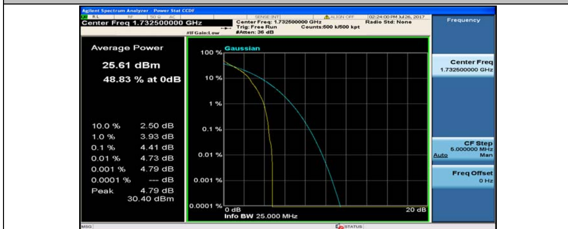
(Channel Bandwidth:15 MHz)_MCH_QPSK_1RB#74
