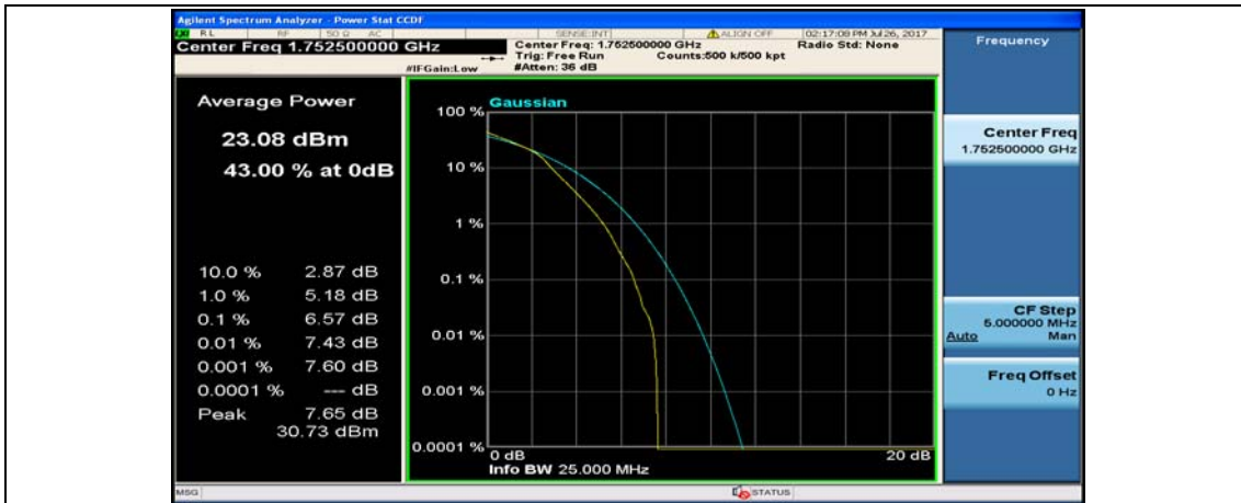
(Channel Bandwidth: 5 MHz)_HCH_16QAM_12RB#13
