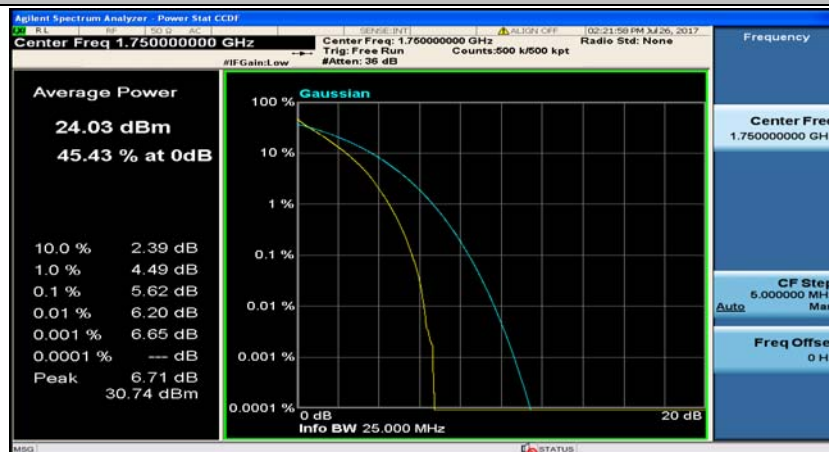
Channel Bandwidth: 10 MHz_HCH_QPSK_50RB#0
