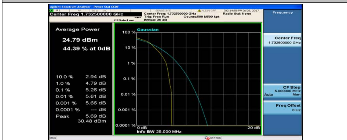
(Channel Bandwidth: 5 MHz)_MCH_16QAM_1RB#12
