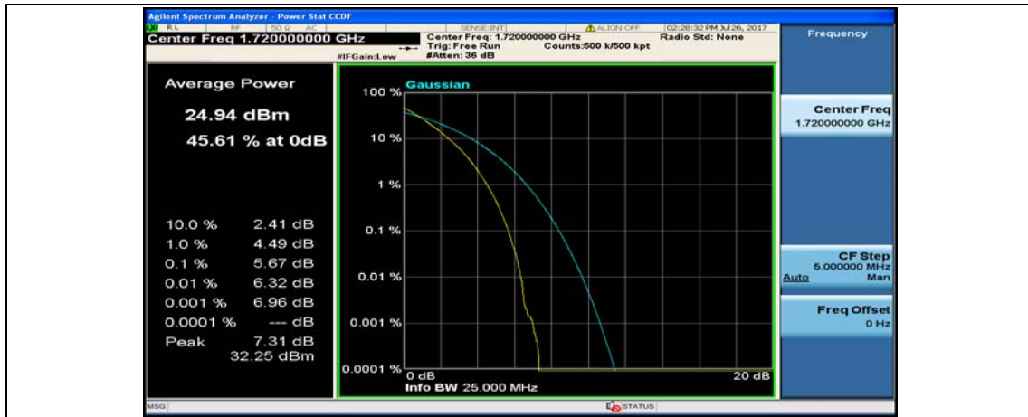
(Channel Bandwidth:20 MHz)_MCH_QPSK_1RB#0
