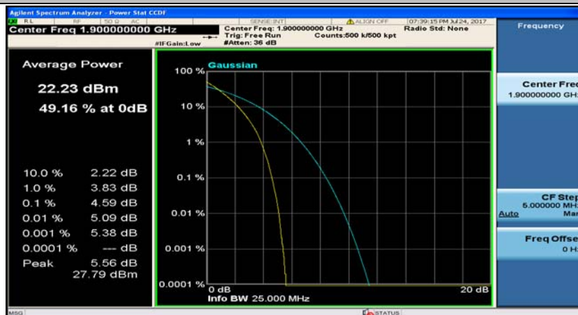
(Channel Bandwidth:20 MHz)_HCH_QPSK_100RB#0
