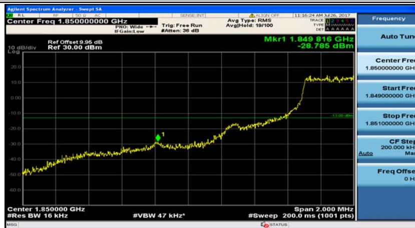
(Channel Bandwidth: 1.4 MHz)_LCH_QPSK_6RB#0
