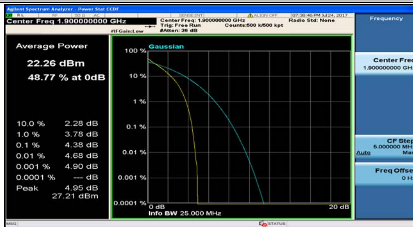
(Channel Bandwidth:20 MHz)_HCH_QPSK_100RB#0
