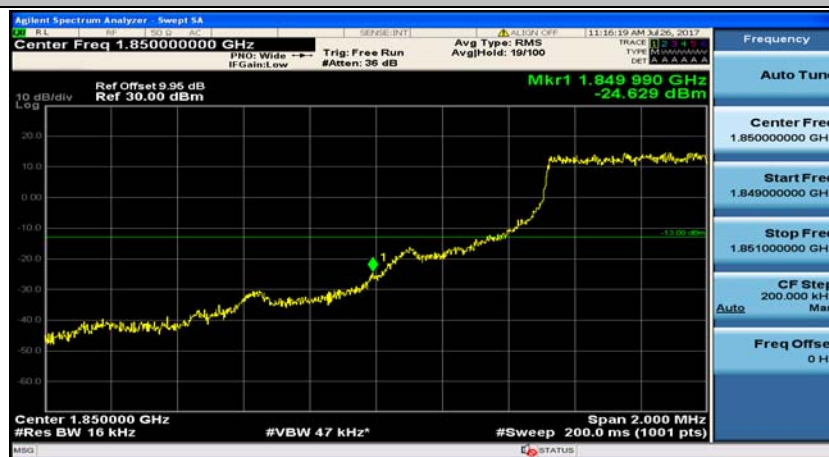
(Channel Bandwidth: 1.4 MHz)_LCH_QPSK_3RB#3
