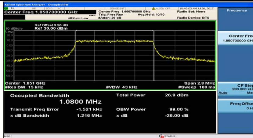
(Channel Bandwidth: 1.4 MHz)_LCH_16QAM_6RB#0
