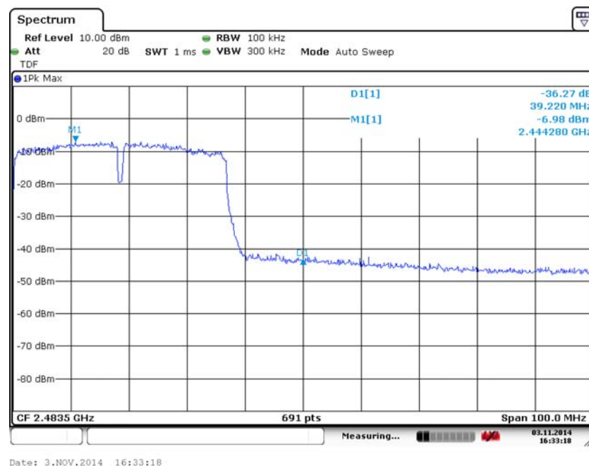
Fig. 116 Band Edges (802.11 n-40MHz, Ch 9)
