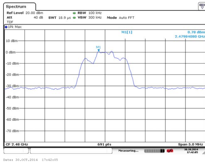
Fig. 37 Conducted Spurious Emission ( \pi/4 DQPSK, Ch78, 2.480GHz)
