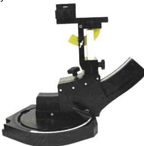
Device holder supplied by SPEAG
