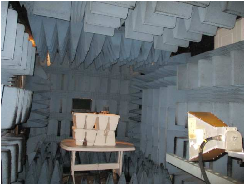
Figure 9. Band Edge screening set up, "dipole" antenna
