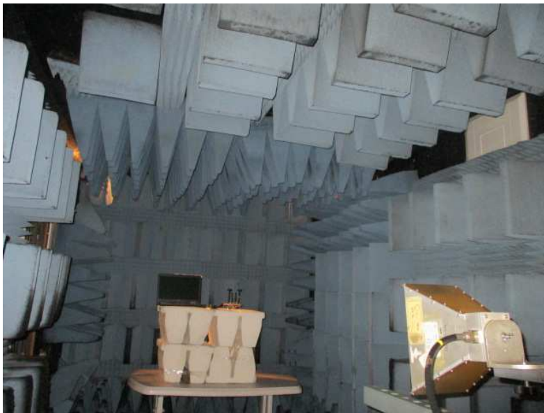
Figure 8. Band Edge screening set up, "mushroom" antenna
