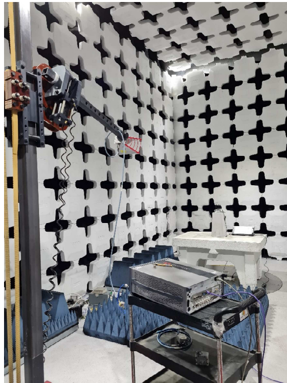
Figure 11. Radiated Emission Test, 12-15GHz
