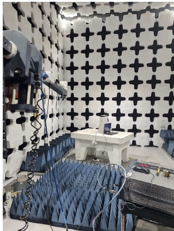
Figure 12. Radiated Emission Test, 15-40GHz
