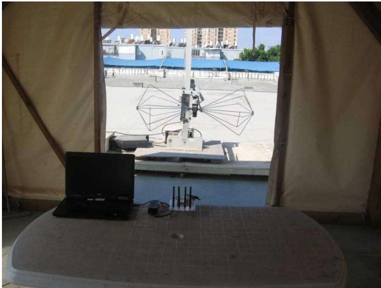
Figure 6. Radiated Emission Test, 30.0-200.0MHz
