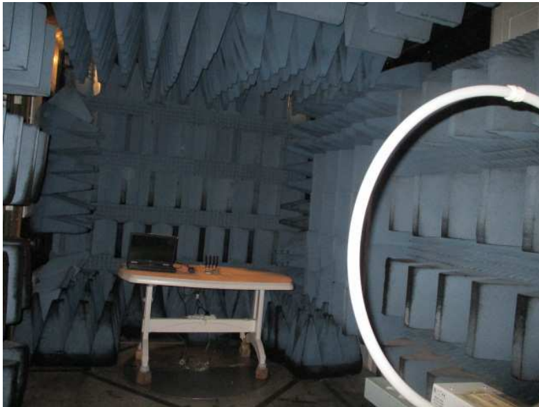
Figure 5. Radiated Emission Test, 0.009 30.0MHz
