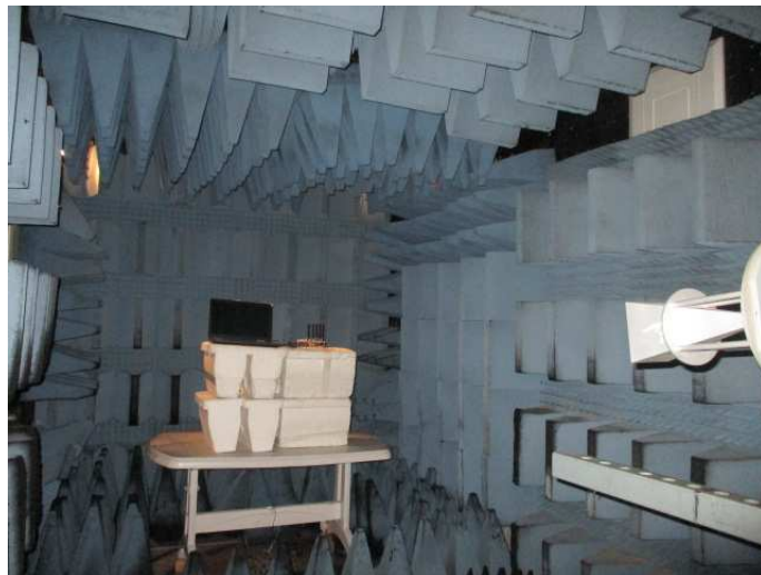
Figure 6: Radiated Emission 18GHz – 26.5GHz
