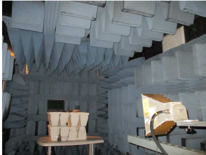
Figure 5: Radiated Emission 1GHz – 18GHz
