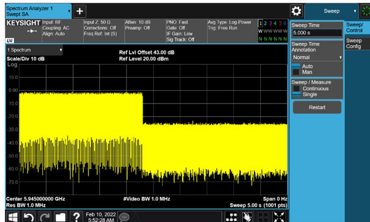
Figure 72. EUT evacuation of frequency 5945.0MHz (40.0MHz BW) due to incumbent signal at 5960.0MHz
