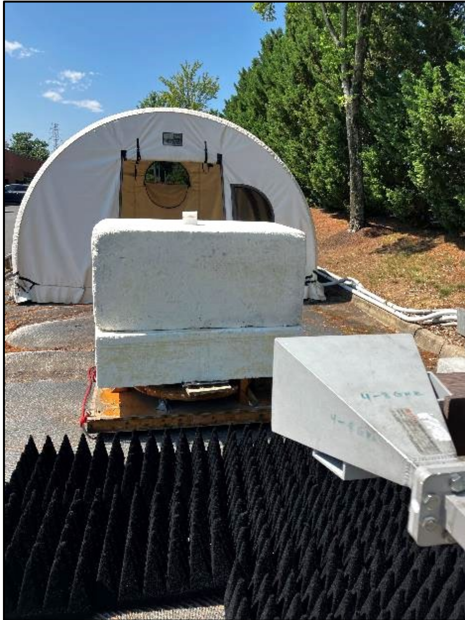
Photograph 2: Radiated Emissions Testing – Back View, Greater Than 1 GHz
