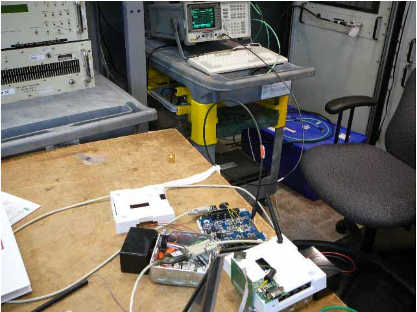
Figure 5 - Radiated Spurious Emissions Test Setup (Semi-Anechoic Chamber 2)
