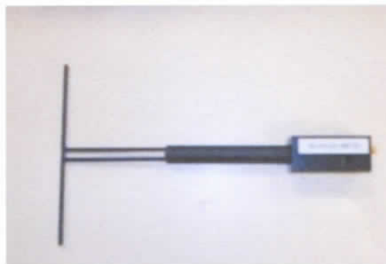
Figure 1 – Satimo COMOSAR Validation Dipole
