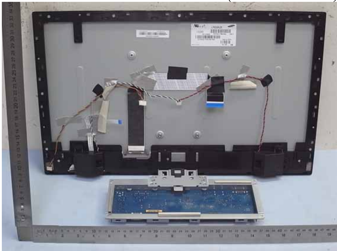
Figure 16 Internal View (Removed Shielded Case)
